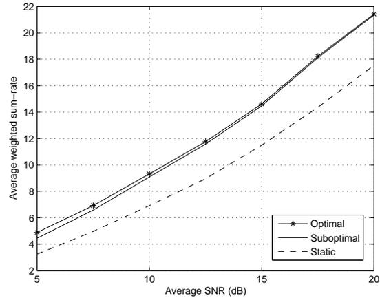
**Fig. 3.** Average weighted sum-rate versus average SNR for optimal, suboptimal and static schemes ( $K = 2$  users,  $N = 8$  subcarriers,  $w_1 = 0.6$ ,  $w_2 = 0.4$ ,  $BER = 10^{-3}$ ,  $P_{tot} = 1$ ).
